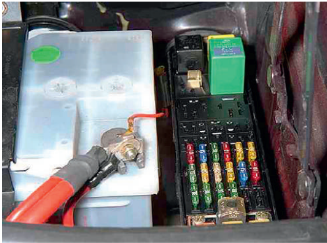
Figure 3.51 Correct polarity is important: red cables are used for the positive connection
